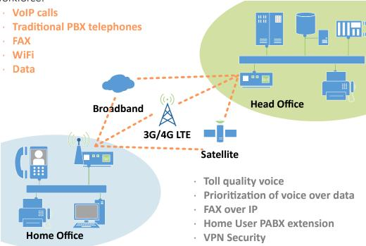
Interoperability is a key element of the VoLTE VoicePAC family, which means that the devices can be integrated with existing TDM based PBX, soft switches, IP based telephony and IP data networks. Data and voice can be handled together with user definable prioritisation ensuring that the toll quality of voice communications can be maintained no matter what the load.
